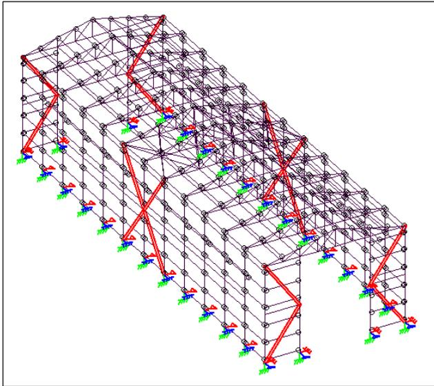
**Fig 5: Single Diagonal bracing (center)**
