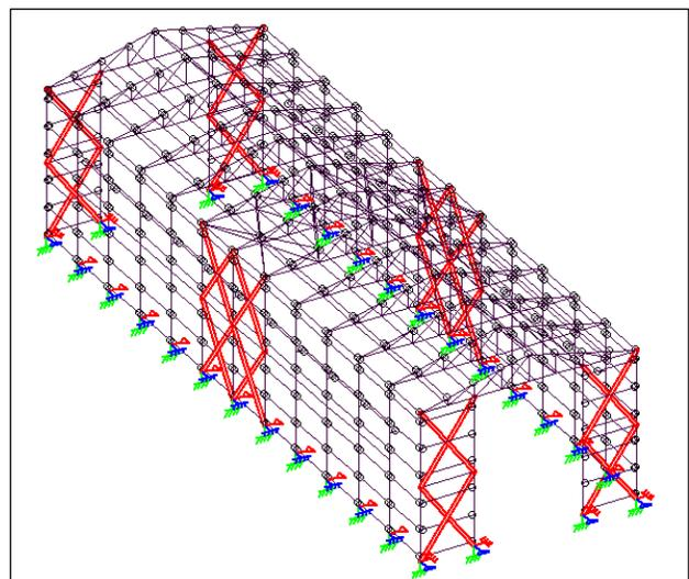
**Fig 3: X bracing (center)**
