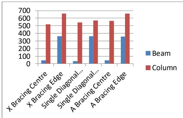
Fig 10: Graphical representation of Maximum Beam end Forces
