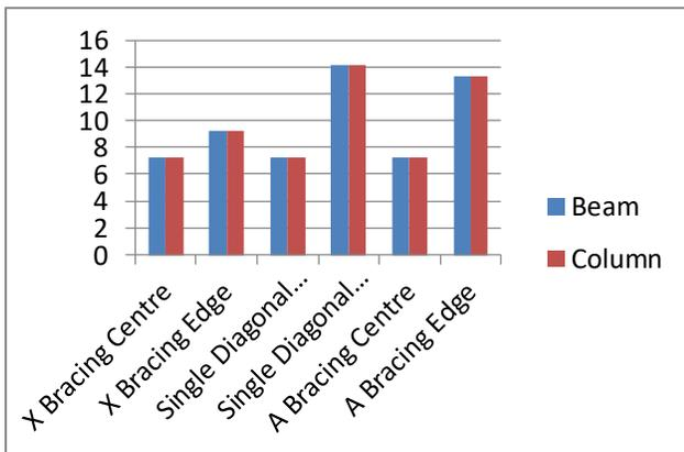
Fig 9: Graphical representation of maximum displacement
