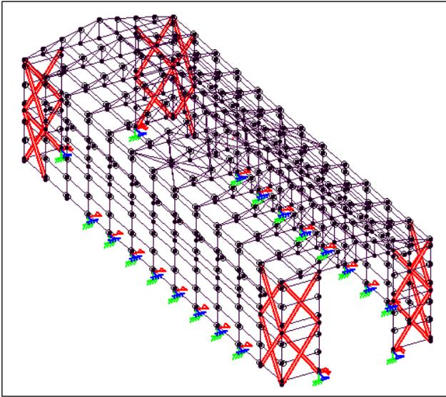
**Fig 4: X bracing (Edge)**
