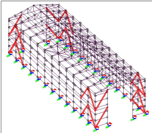
**Fig 8: X bracing (Edge)**
